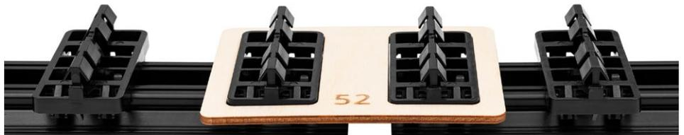
PaCS Alu Rail Start must be screwed to the substructure every 400 mm. Always ensure that all rows of clips are in perfect alignment before fixing PaCS CLAD or PaCS Alu Rail to the wall substructure.
